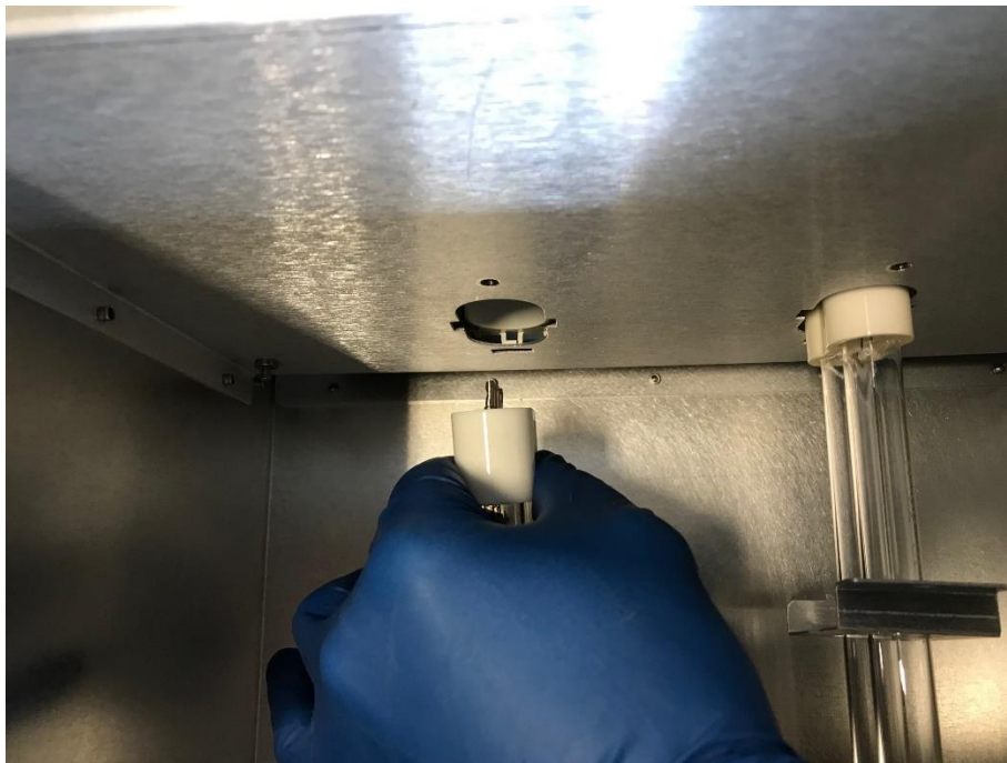
Figure 12: Carefully Pull at Ceramic Base to Remove Bulbs
