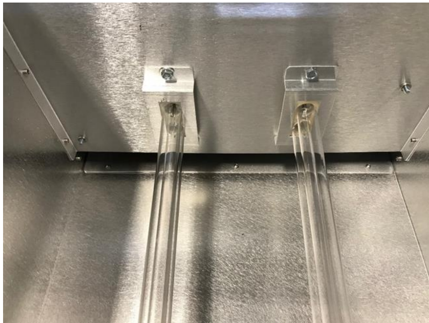
Figure 13: Install New Bulbs, Bulb Support Clips and Bulb Support Wire
