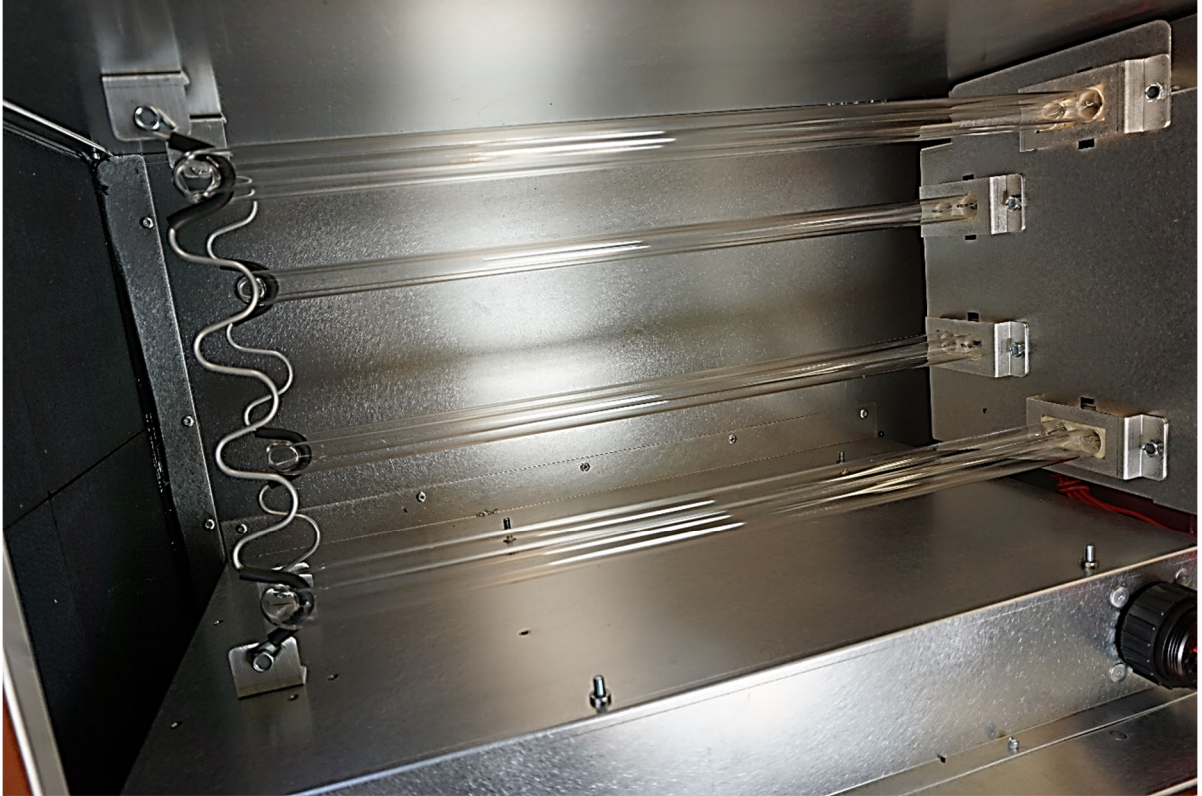
Figure 14: Completed Bulb Assembly
